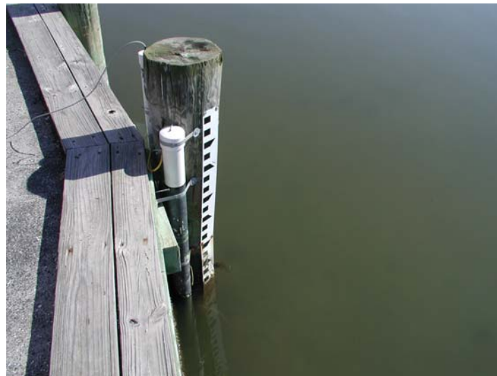
Figure A-6. The water level sensor is mounted in the bottom of a stilling well consisting of a 5-foot length of 3-inch PVC pipe. Also shown is a 5-foot tide staff. The water level is the photograph is approximately 2.2 feet.
