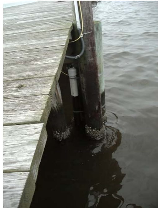
Figure A-9. The stilling well containing the water level sensor was attached to a support piling next the light pole. Water depth is approximately 3 feet.
