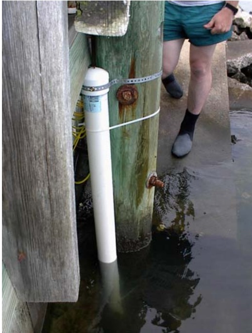
Figure A-2. The stilling well was mounted on a piling and the recorder box (GL400) was placed under ornamental grass plantings (shown in photo to the right). The water depth at this location is approximately 2 feet.
