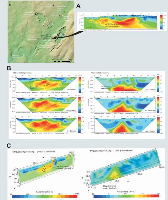
Figure 7. Resistivity at Albert Powell. A. LIDAR-derived location map of ER surveys relative to the Hatchery and dye injection sites. Profile of ER survey 1 showing highly resistive anomaly. B. Expanded ER and IP surveys 50 meters north of ER Survey 1. A resistive zone (red in ER images to left) occurs above a highly chargeable zone (red in IP images to right). C. Quasi-3D processing of ER (left) and IP (right) survey lines 1-3.
