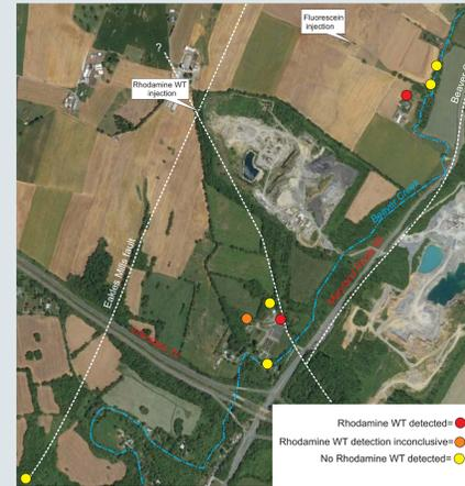
Figure 5. Google Earth image of Albert Powell Hatchery areas and locations of dye trace injection and monitoring sites.
