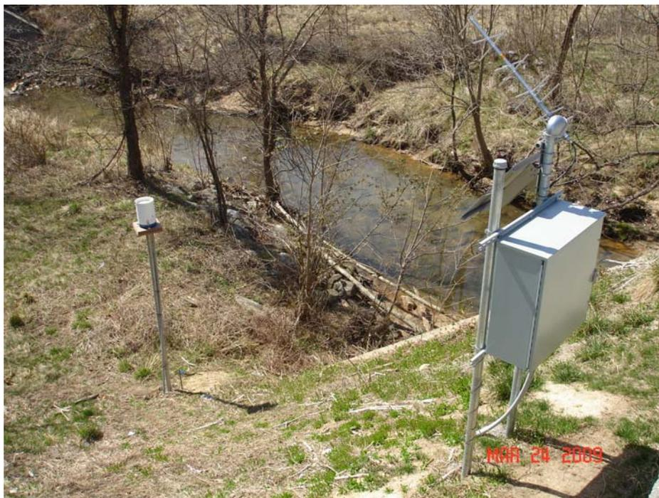
Figure 10. Stream gage and rain gage at Dorsey Run.
