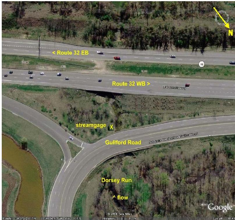
Figure 9. Stream gage (USGS 01594400) on Dorsey Run near Ft. Meade between Guilford Road and Rt. 32 bridges. [View is to the southwest]
