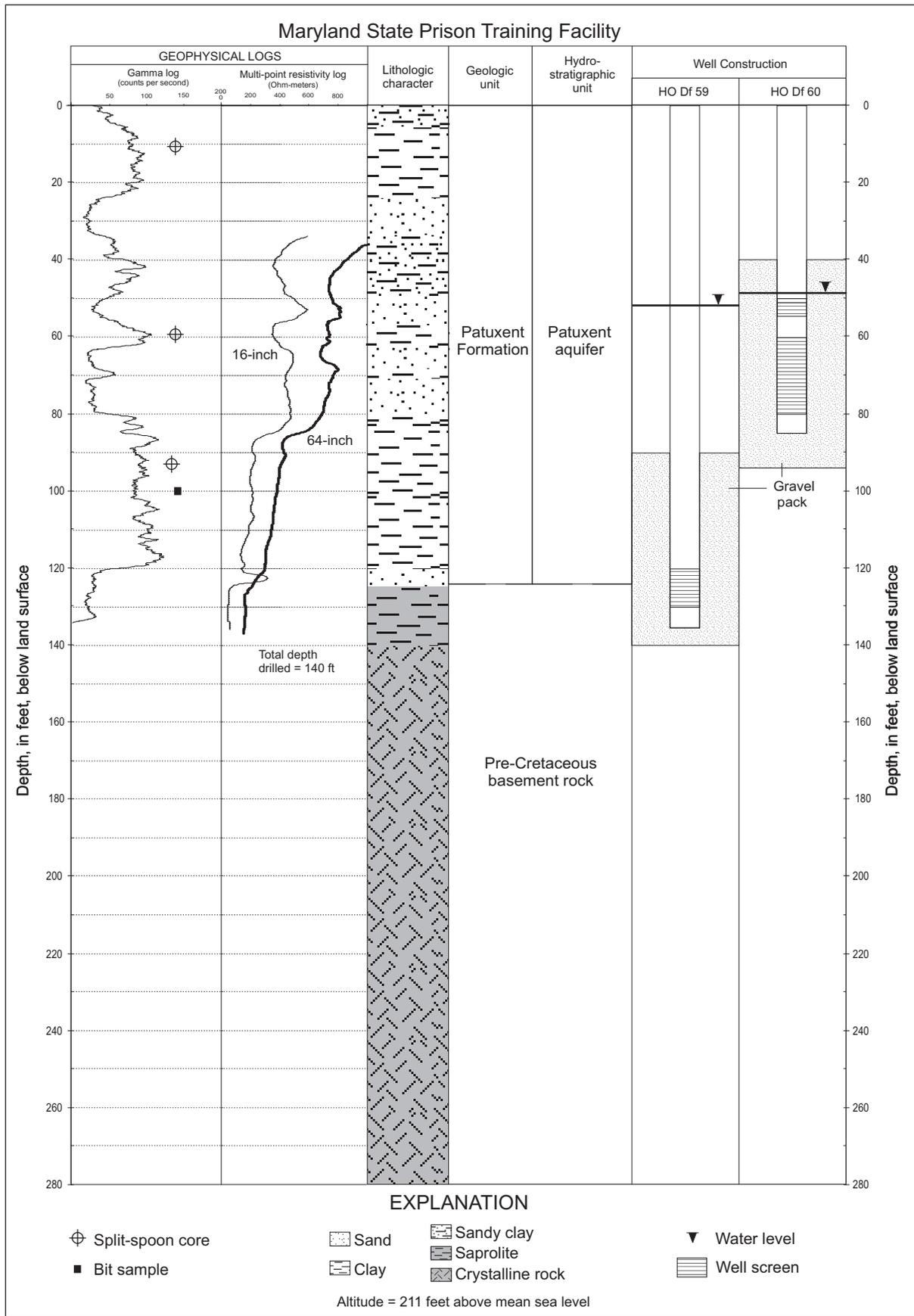
Figure 3. Geophysical, geologic, and hydrogeologic data from test wells.
