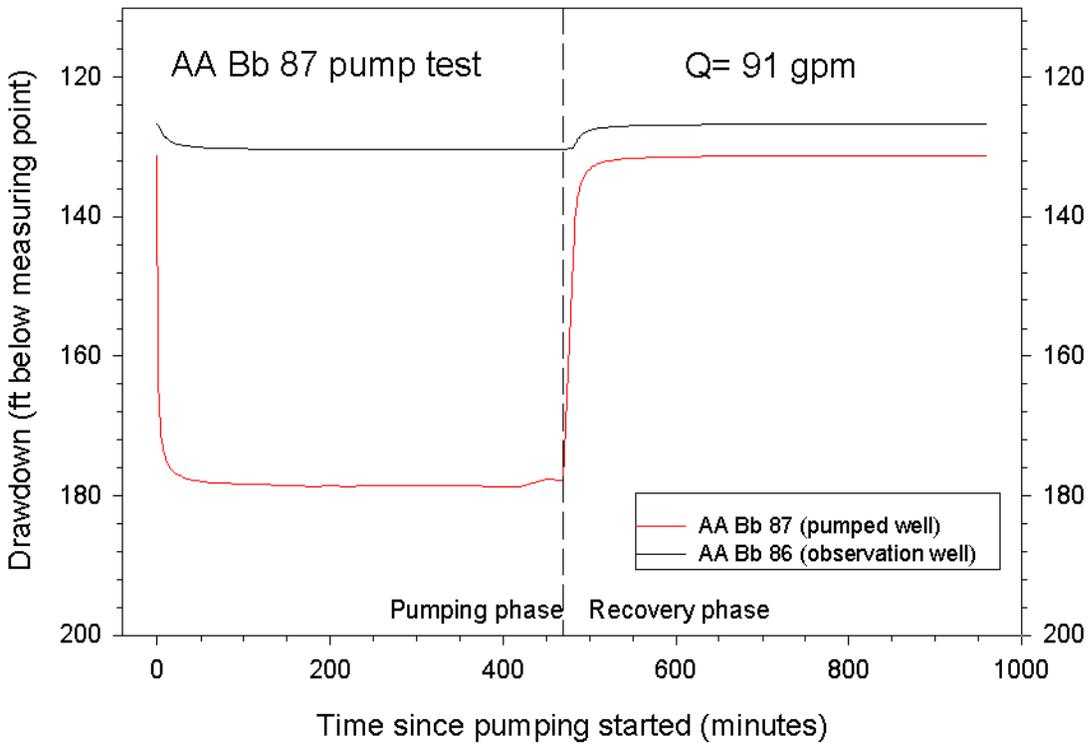
Figure 5. Drawdown and recovery data from pump tests in paired wells.
