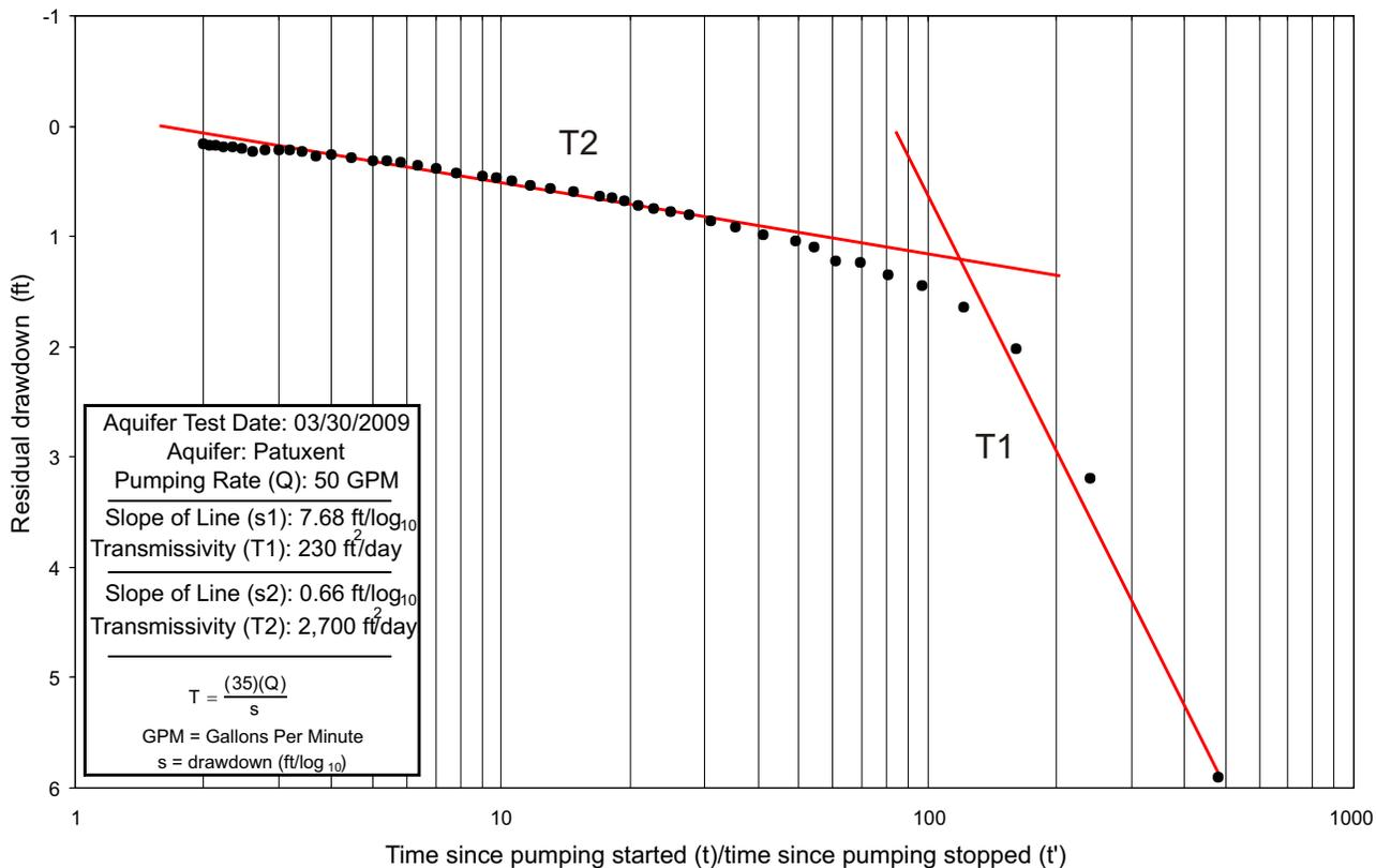
Figure 4. Drawdown and recovery data and transmissivity calculations for test wells.
