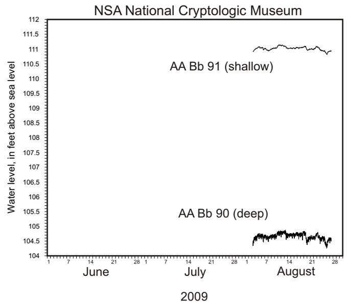
Figure 6. Hydrographs from test wells.
