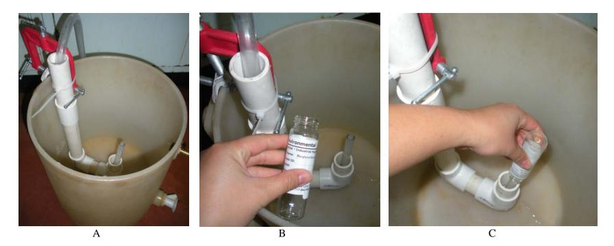
Figure 8. Inverted bottle technique for dissolved-methane collection of well-water samples. Step A: Clear tubing is connected to untreated water source (e.g., pressure tank spigot), and the water is turned on to fill up the sampling bucket. Step B: Cap is removed from glass vial. Step C: Glass vial is inverted and placed over the clear tubing. Water fills the vial and is allowed to flush three vial volumes before the vial is capped underwater (modified from Hirsche and Mayer, 2009).
