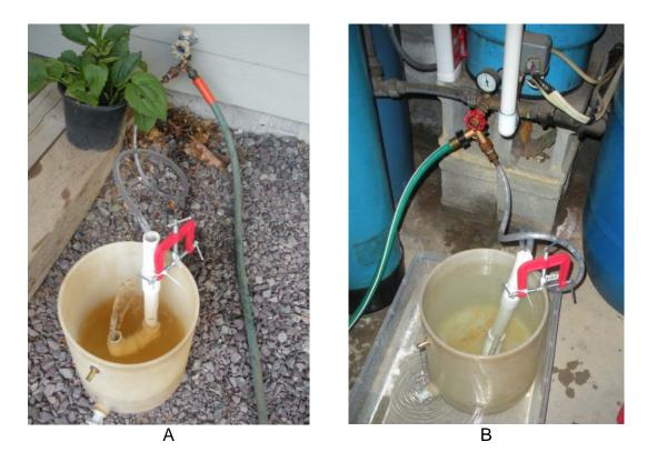
Figure 7. Photographs showing different sampling ports for dissolved-methane collection. Water treatment systems, if present, were bypassed during purging and sampling.
