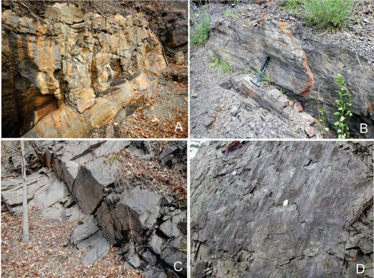
Figure 16. Rock friction. A, Rough and irregular. B, Undulating. C, Planar. D, Slickensides.
