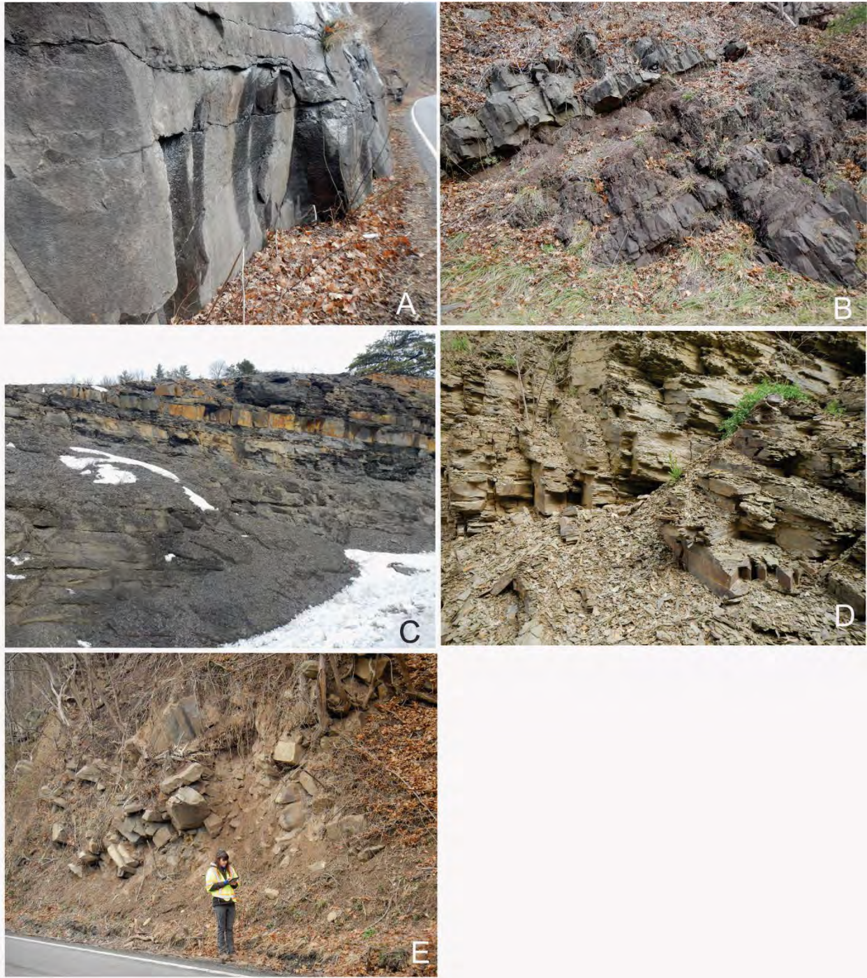
Figure 20. Lithology. A, Massive sandstone/limestone. B, Sandstone/limestone with shaly interbeds. C, Shale with sandstone/limestone interbeds. D, Massive shale. E, Block in matrix.
